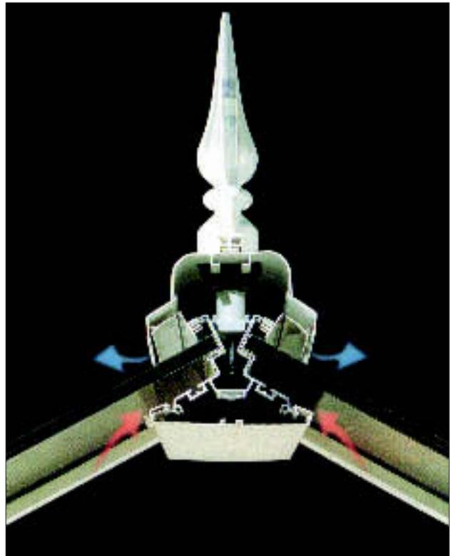
Figure 8 Speedloks clamped to glazing bars, which are fixed to the die-cast ridge end
