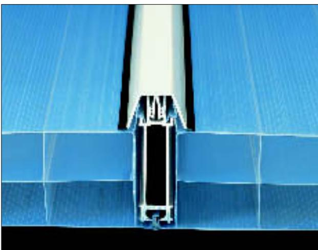
1.6 The glazing panels are joined together by aluminium interlocking reinforcing bar sections extruded from aluminium to BS 1474 : 1987, material designation 6063-T6, with PVC-U external claddings and TPE co-extruded gaskets.
