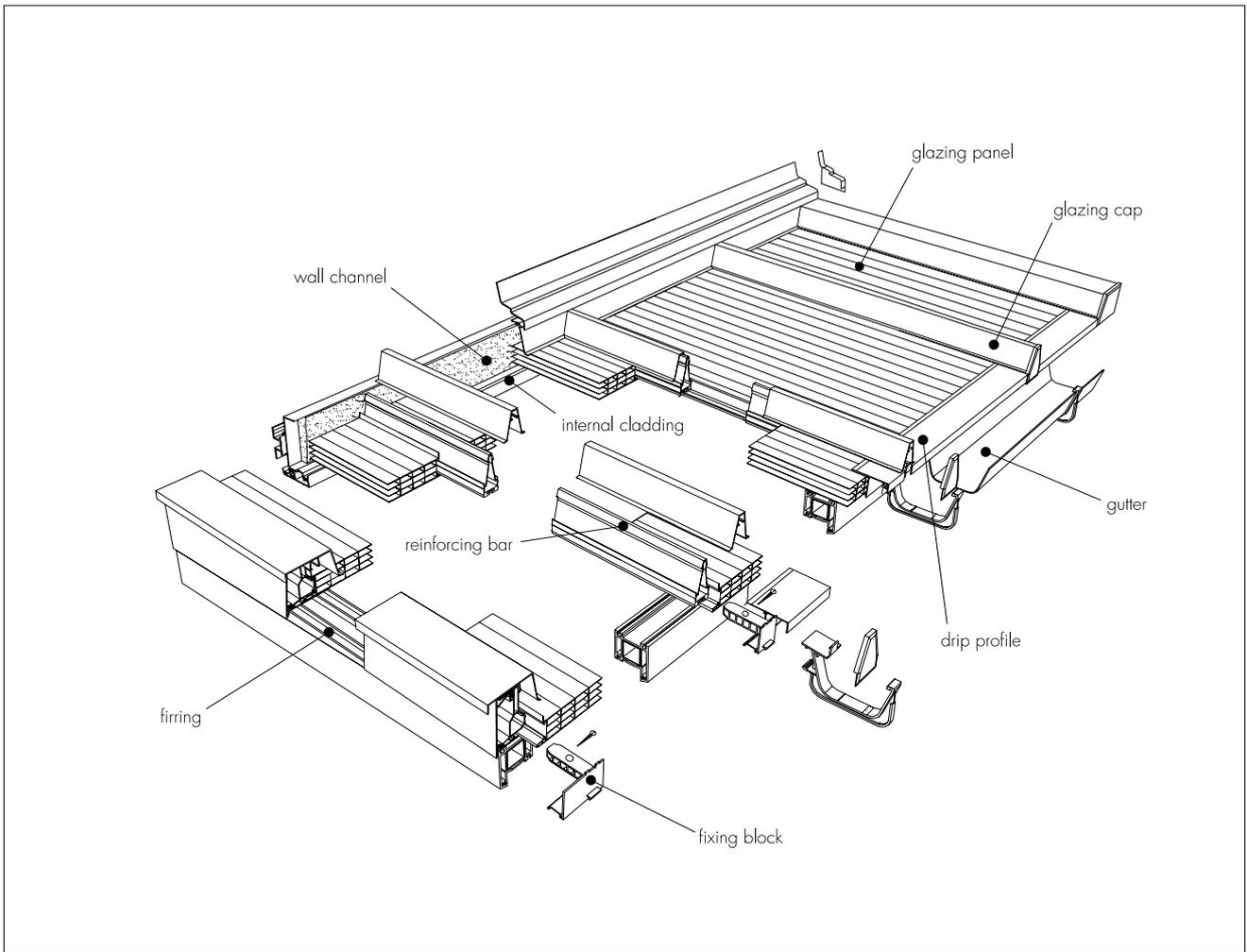
Figure 3 Section through Ultralite 500 PVC
