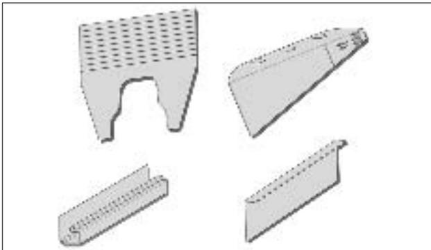
1.16 For duo-pitched roofs, stepped flashing panels (left and right) slot into a preformed soaker which is pre-clipped into the starter bar of the roof (see Figure 5). A saddle apron panel and horizontal flashing is used at the apex.
