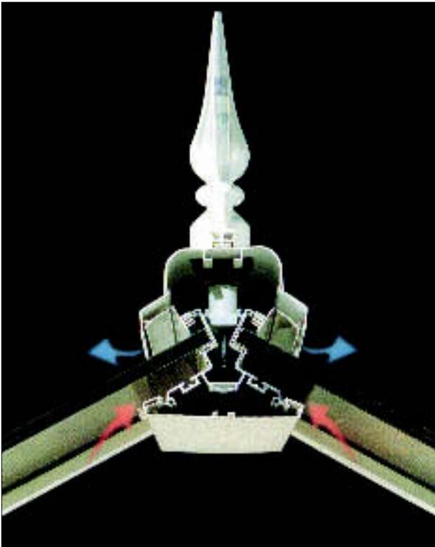
Figure 8 Speedloks clamped to glazing bars, which are fixed to the die-cast ridge end
